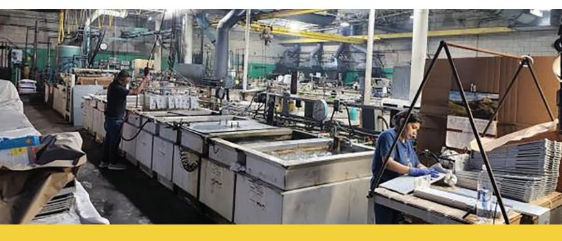
ZINC PROCESSING LINE AND VARIOUS METAL PROCESSING EQUIPMENT
